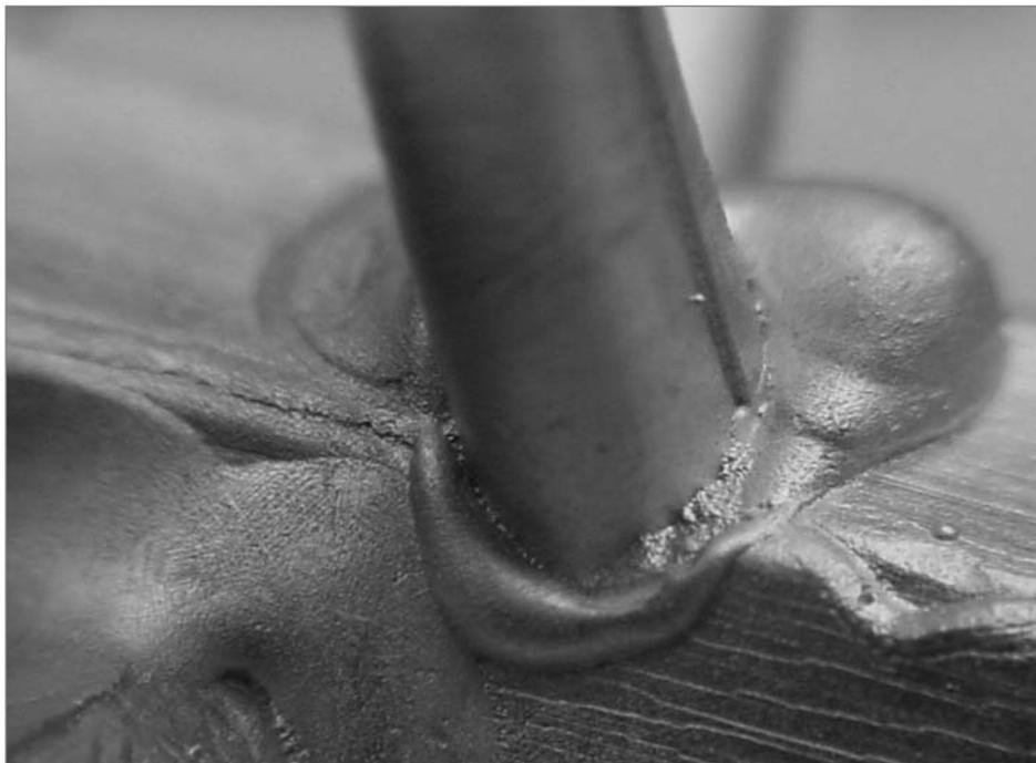
*Figure 9 Gate/sprue interface 1*
